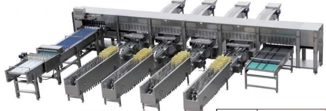
• Constructed from high quality stainless steel for great durability and hygiene. • Equipped with colour touchscreen PLC control and self-diagnose system and can sort eggs into 4 grades with accuracy $\pm$ 1g.
