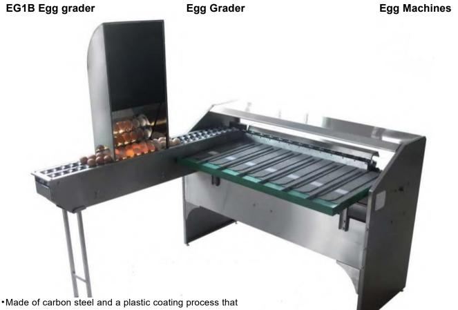
•Made of carbon steel and a plastic coating process tha enables greater durability.
